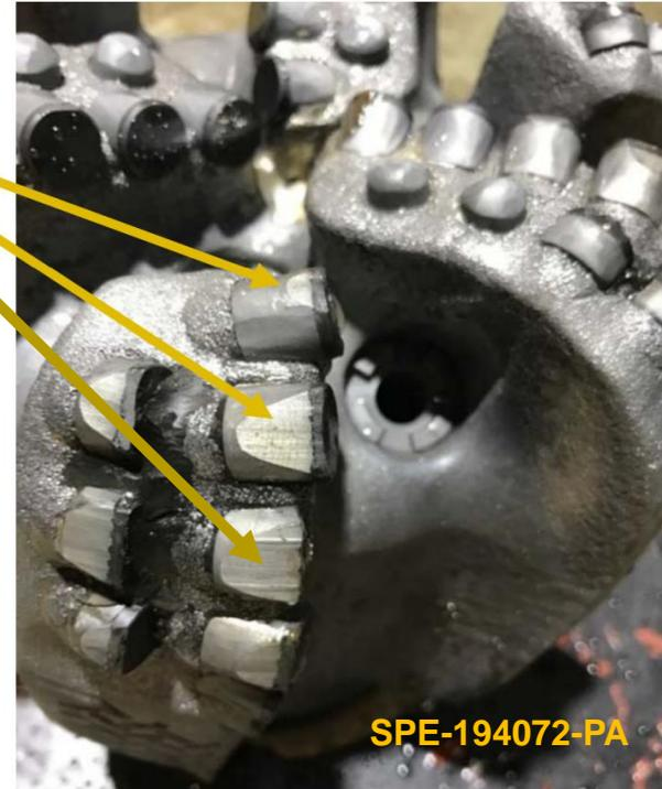
Fig. 4—Post-run pictures of the bit for the run that resulted in the twistoff.
